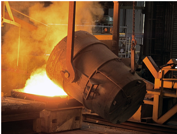
Figure 11.5 Traditional thin casting in mold with silicon fines (Møll, 2014).
