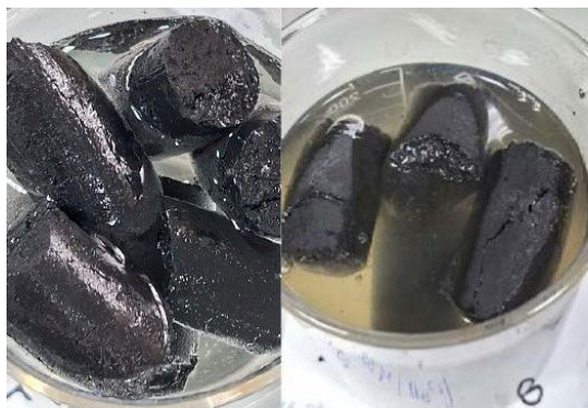
Figure 4: Water-resistance test: extruded charcoal briquettes after five days of full immersion in distilled water, with no visible disintegration of the cylindrical agglomerates.
