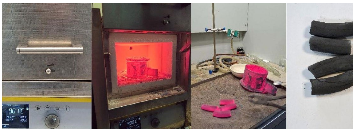
Figure 5: Thermal-shock test sequence: muffle furnace at 900 °C (left), briquettes in the sealed oxygen-free container during heating (centre-left), the container during cooling (centre-right) and the briquettes after cooling with shape retention (right).
