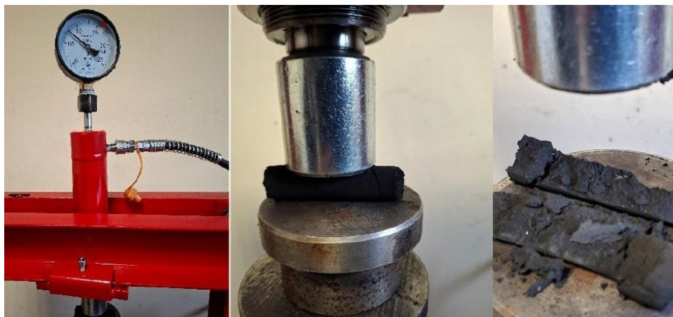
Figure 2: Compression test on the extruded charcoal briquettes: hydraulic press with pressure gauge (left), briquette under axial load (centre) and broken sample after failure (right).
