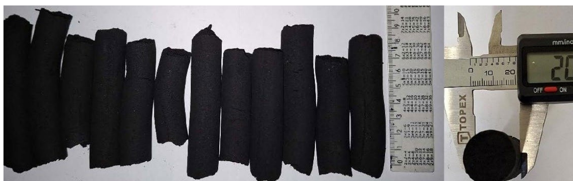
Figure 1: General appearance of the extruded charcoal briquettes and calliper verification of the nominal 20 mm diameter.
