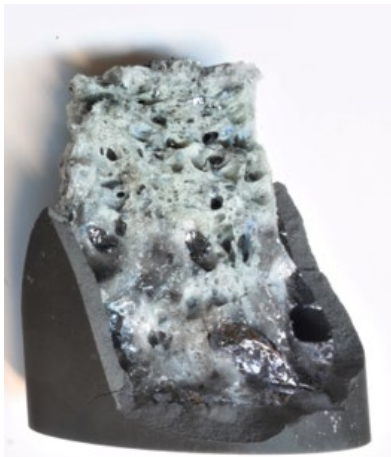
Figure 7 Crucible after experiment at 1800^\circ\text{C} showing segregation with Si at bottom with melted \text{SiO}_2 above. Diameter of crucible is 42 mm.
