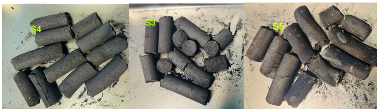
Figure 19. Visual aspect of pellets after shock heating at 500 °C.
