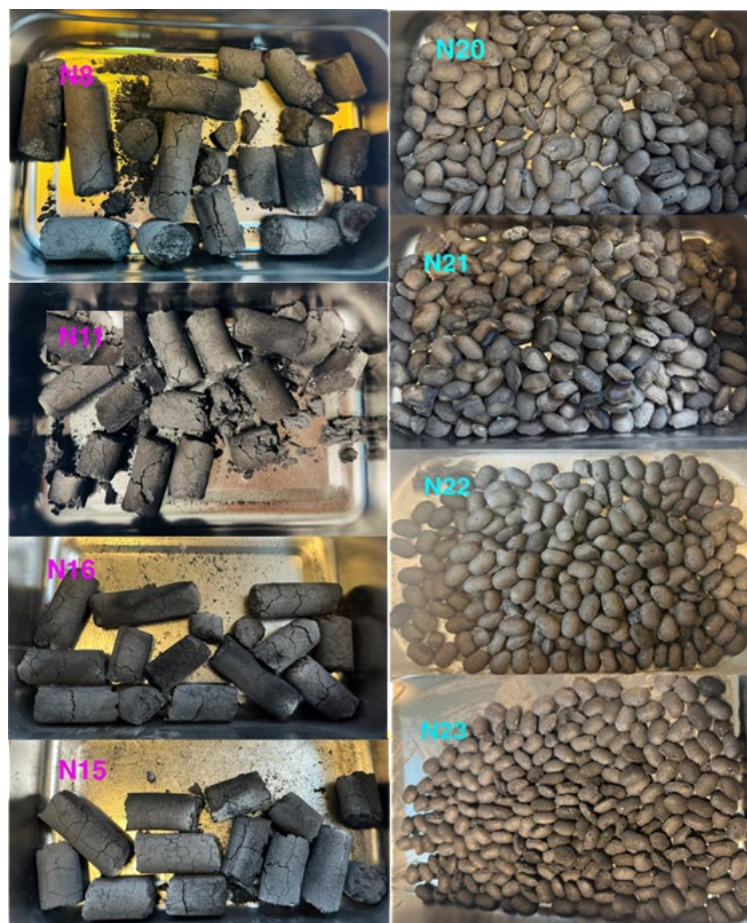
Figure 18. Visual aspect of pellets and briquettes after shock heating at 1000 °C.
