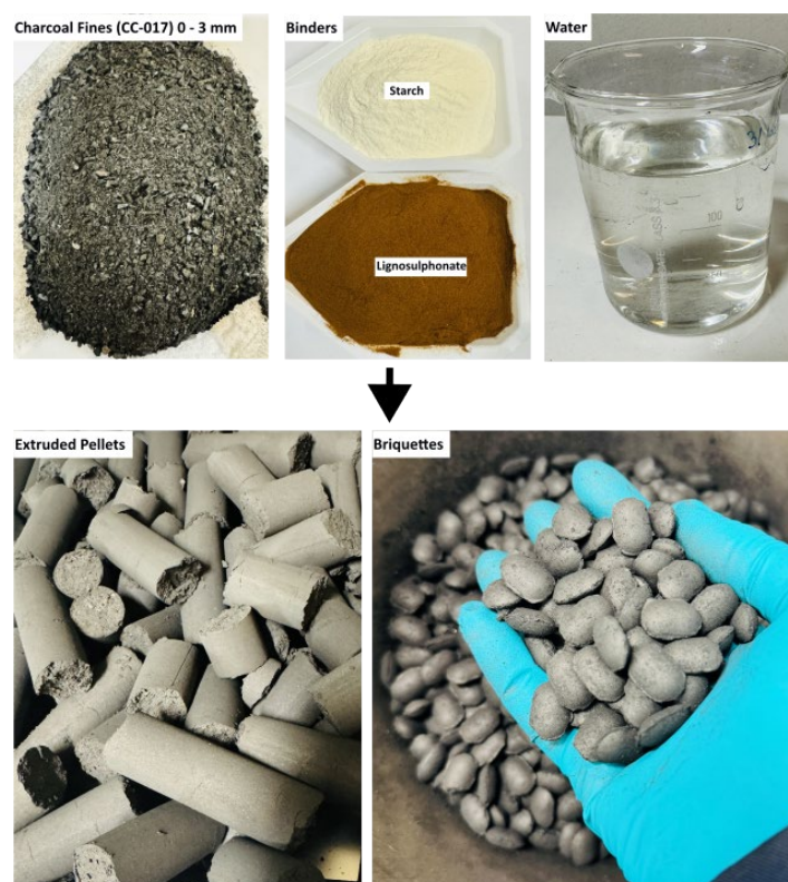
Figure 1: Raw materials used for producing charcoal pellets and briquettes
