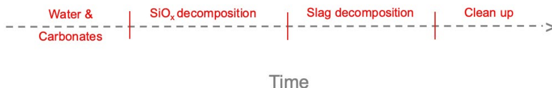
Figure 1: Schematic representation of oxygen-containing species decomposition during temperature ramping
