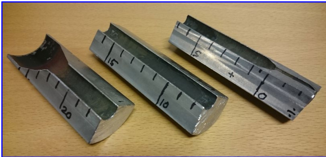
Figure 4: The pieces of the reactor that was examined by SEM. Pieces from left to right is from top to bottom
