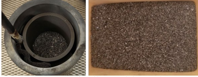
Figure 4 Image of crucible setup and silicon sample.
