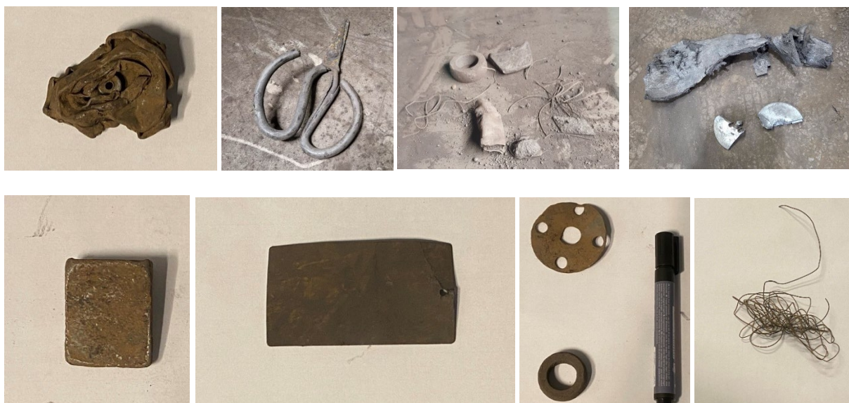
Figure 7: Pictures showing samples of fragments found in the kerf raw material. Scale approximately 1–5 cm.
