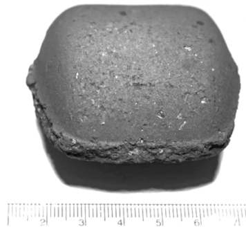
Figure 3. Charcoal briquettes with cornstarch binder used in trials
