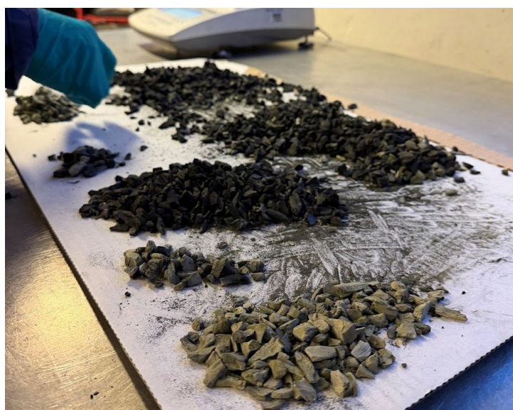
Figure 2: Sorting degree of SiC conversion from charcoal/coal manually by colour. The green/grey material closest to the camera is the most converted SiC.
